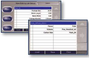
**Nested Recipes** can be downloaded as a data source, allowing InteractX to manage/edit detailed Recipes and formulations, which can also be shared with multiple machines running Xpress.
